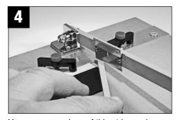
You can use a piece of thin stripwood as a spacer between the fence and the angle gauge to move the strip being cut away from the fence.
