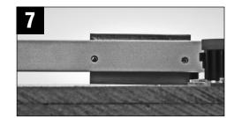
For better cutting action, the blade is deliberately set at a slight angle to the base board to provide a slight slicing action. Be sure to press down far enough to completely cut through the workpiece.
