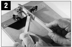
Use Chop-It as shown above to cut stripwood at an angle. Note: Large angles will increase the effective width of cut; avoid overloading the tool by attempting to cut thick pieces at a large angle.
