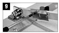
If the cutting pressure increases, the blade is getting dull and needs immediate replacement. Loosen one blade-retaining screw, then remove the other. Now remove the blade. Be careful...do not cut yourself! Blade installation is the reverse of removal.
