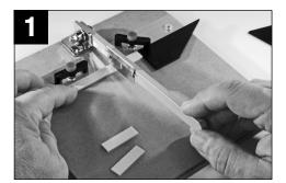
Use Chop-It as shown above to cut a set of stripwood pieces to the same length. Use the right-angle gauge as a stop bar.
