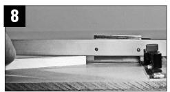
Do not attempt to cut materials thicker than the blade protruding from the bottom of the handle (about 3/16 inch); otherwise the handle will strike the top of the workpiece before the blade has a chance to cut all the way through it.
