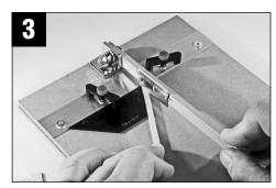
Use the angle gauges for common angles. Position the gauge so it clears the cutting edge of the blade. Use the locking clamps to hold in position.
